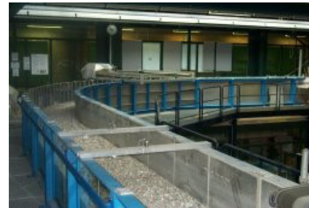
Figure 5.16. Curved channel (25 m x 1 m) and channel with variable slope (43 m x 2 m).
