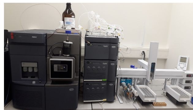
Figure 5.14. Liquid chromatography tandem mass spectrometer (LC-MS/MS) used for the analysis of various organic compounds.
